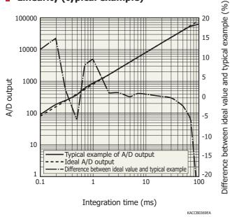
A/D output is the output with dark output subtracted when light is input. The difference between the ideal value and typical example contains a measurement error. The smaller the A/D output, the larger the measurement error.
