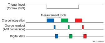
In any of the modes 1 to 6, if the trigger input cycle is shorter than the measurement cycle of the spectrometer, the input trigger is ignored.
